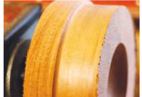
▲ The finish from the Easy Wood tool on the left of the blank isn't as clean as the right, which was completed using a bowl gouge
